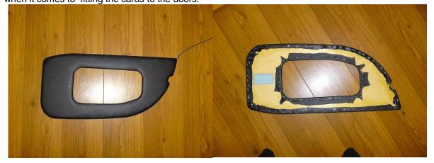
I cut pieces of material for the curtain effect map pocket and the centre of the door card. The map pocket should be cut approx 50% wider than the centre space.
