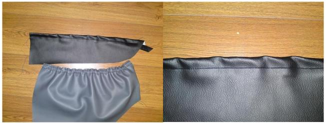
I used a metal ruler to fold the vinyl over twice (a French seam so I'm told) and clipped it in to position. I then ran a stitch 10mm across the top followed by a 24mm stitch. This created a nice channel to thread the elastic through. I stitched the elastic in to the channel at on end pulled it taught and stitched at the other end. Giving a nice curtain.
